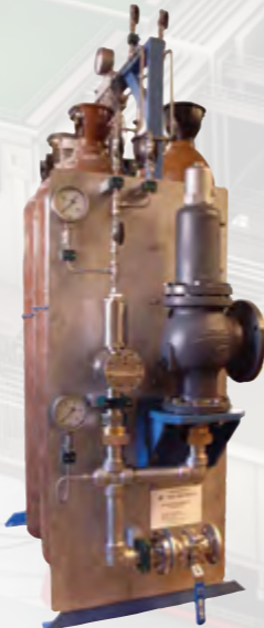
Hale Hamilton's Flare Gas Purging Panel utilises the RH25 Dome Loaded Regulator and F105 Filter. The panel introduces nitrogen to the flare gas supply line to snuff out the flare or to purge the flare stack.
